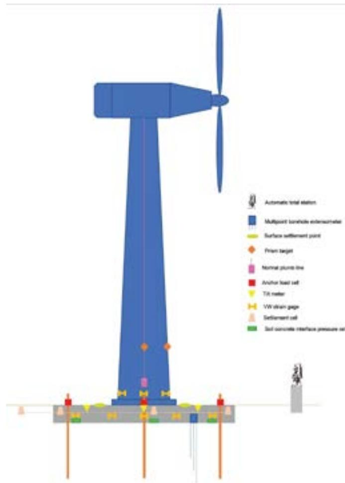
Typical instrumentation scheme of a wind turbine
