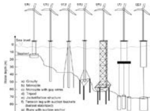
Types of foundations of on shore (left) and off shore wind turbines (right)
