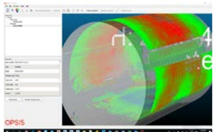
DEFORMATION MONITORING USING OPSIS SOFTWARE
