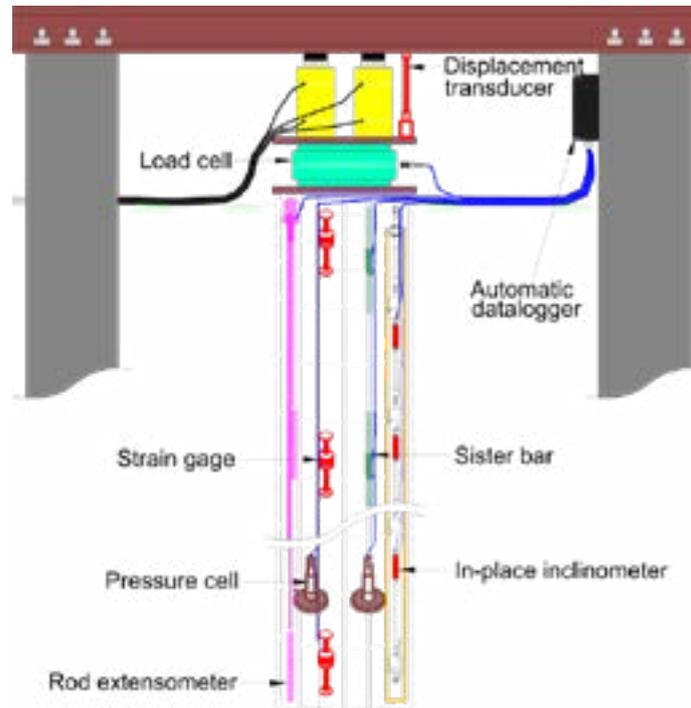
Typical instrumentation scheme of a wind turbine pile foundation testing
