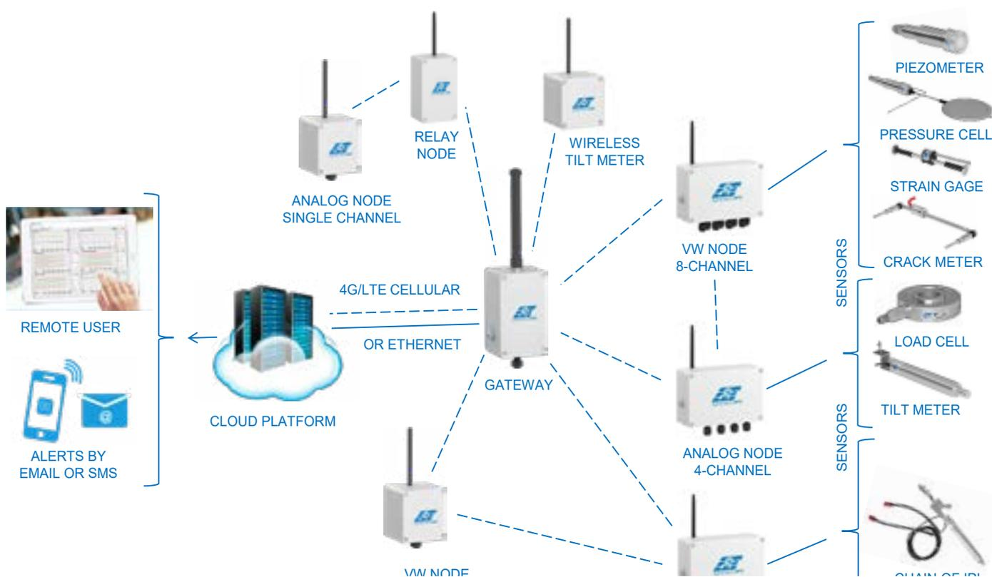
Remote real-time monitoring system with wireless (RF) nodes and gateways
