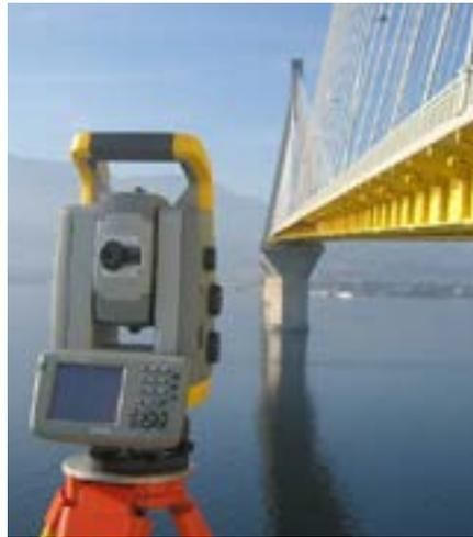
STRUCTURAL MONITORING USING ATS
